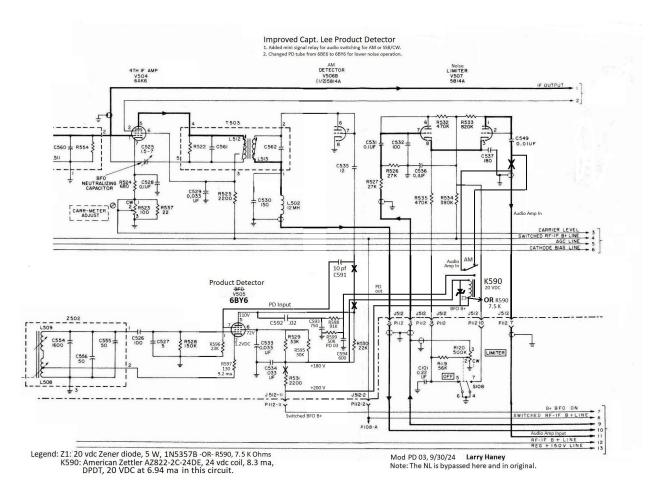
You will notice that there is a 20 VDC Zener diode across the relay coil. This stabilizes the voltage variations that may occur due to AC power for the RX being other than 115 VAC, tube differences or tube aging. But, a 7.5K ohm resistor works very well in its place.
