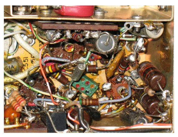
To accomplish the audio switching, I disconnected the white wire with the green tracer from capacitor C549 (which is at the top of the photo mounted on the left side of the circuit board). You can see the wire reconnected to the relay common contact (on the right side of the relay) and an orange wire with white tracer connected to the normally closed relay contact connecting to C549. This is shown in the next photo:
