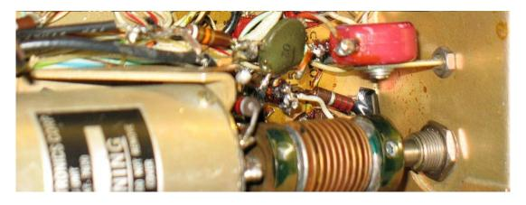
The R531 is changed to 7.5 K in order to apply the correct voltage to the relay coil. This value sets it at about 20 VDC. That is very good for this 24 VDC relay coil, as a much lower value operates the armature and more than 24 VDC will cause it to overheat.
