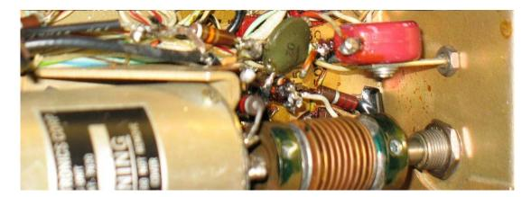
The R531 is changed to 7.5 K in order to apply the correct voltage to the relay coil. This value sets it at about 20 VDC. That is very good for this 24 VDC relay coil, as a much lower value operates the armature and more than 24 VDC will cause it to overheat. That's all there is to using a relay to switch the audio. Have fun.
